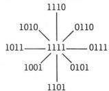
15 (1111) equals stick in the upright (neutral) position. See *Micro*, December 1981, for an article on making a proportional joystick. For an example of a machine language joystick driver you can add to your BASIC program, see **COMPUTE!**, July 1981.
